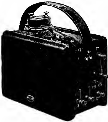
FIG. 253.—A lineman's testing outfit, including telephonic, signaling and battery apparatus.
